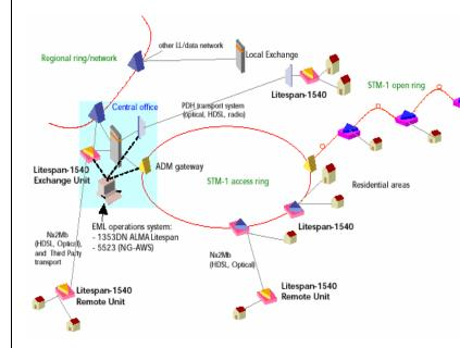
Figure 1: Litespan 1540 in communications network
